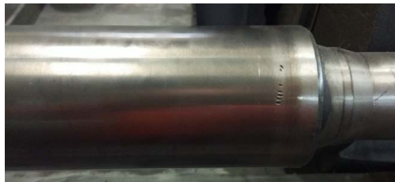
Figure 8. Wear on Work Roll
